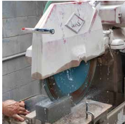
Figure 4. Saw cutting a paver to comply with the aspect ratio (thickness/width) requirements in ASTM C140.
