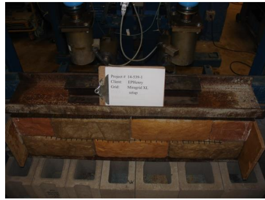
Figure 6 – Placement of Neoprene Pad, Steel Plates, and Steel Beam
