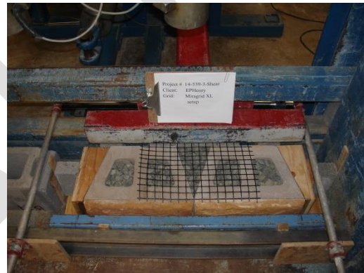
Figure 4 – Placement of Geosynthetic
